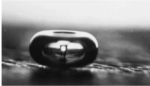
Fig. 2.2 Cavitation jet developed in a single bubble. Reproduced with permission from Crum et al. © IEEE
